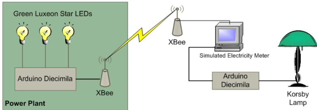
**Figure 11.** Setup of the entire system.
