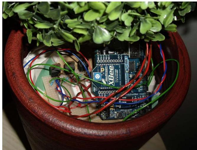
Figure 8. XBee connection inside the vase.
