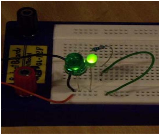
**Figure 14.** 10mm and 5mm LEDs.
