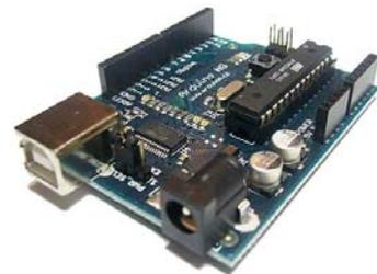
Figure 7. Arduino board.
