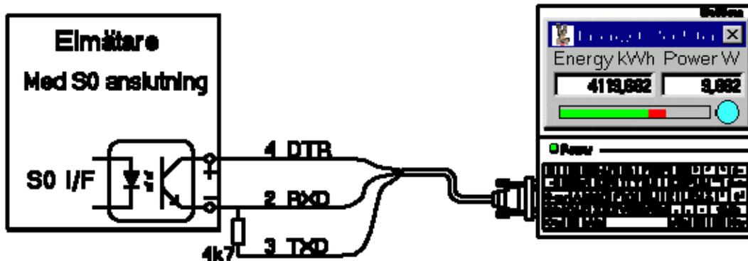
Figure 6. Connection using a cable directly to a COM port.
