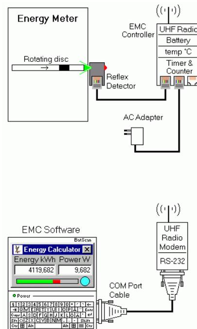
Figure 5. Connection using a radio link.
